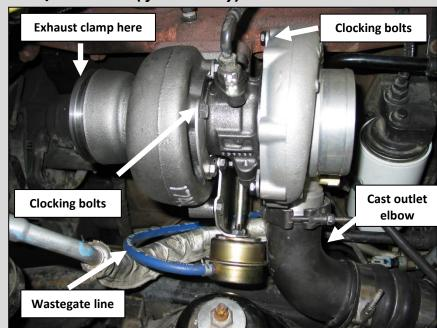
A new compressor outlet O-ring has been provided. Lubricate the O-ring and install between turbo and outlet elbow. Re-use the factory V-Band Clamp. Adjustment of the first intercooler boot may be required for a proper fit.
